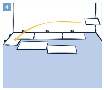
The remaining piece cut off from the last tile in the first row may serve as the first tile in the second row provided it is at least 8" (20 cm) long. Always stagger end joints from row to row a minimum of 8" (20cm) apart.
