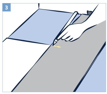
Continue connecting the first row until you reach the last full tile. Fit the last tile by rotating the tile 180° with the pattern side upward, place beside row. Measure and mark, then using a ruler and utility knife, score the tile and snap off. Attach as described above.
