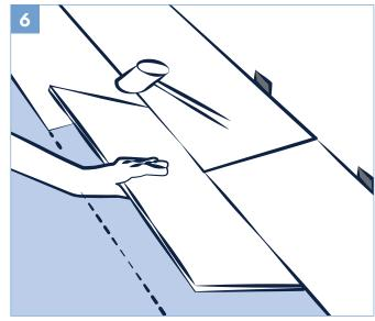
Install the second tile of the second row. Position the long side of the tile with the tongue side, fully engage into the receiver of the first row of product. Lower the tile with firm pressure to the floor, ensuring that the end joint is overlapping and perfectly aligned; push the end joint downward till the end of the tile snaps in place.
