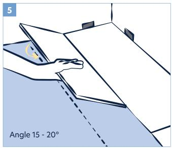
Install the long side of the first tile of the second row. Place a 1/4" (6.35mm) spacer between the wall and the short side of the tile. Insert the tongue side into the groove side of the tile from the previous row at a low angle and lower flat to the substrate.
