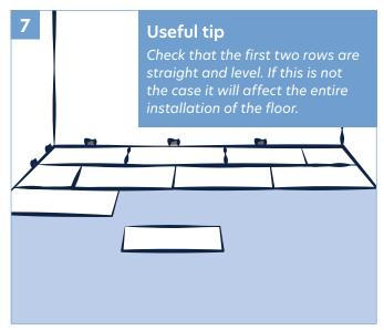
Continue installing tiles in the second row. Continue working from left to right, row by row. Be sure to maintain a 1/4" (6.35mm) space around all walls and vertical objects. To maintain a random appearance, remember to offset end joints a minimum of 8" (20cm).
