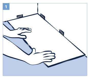
Begin laying tiles from the left side of the starting wall and work to the right side. The tongue of the tile should face the starting wall. Place 1/4" (6.35mm) spacers between the short and long side of the tiles and the wall Always position one spacer between the wall and where the tiles join.
