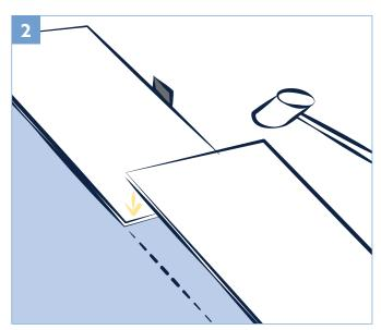
The end joints of the tiles in the first row are assembled by inserting the tongue side into the groove side of the previous tile at a low angle. Gradually lower the tile down flat until the end joint closes, ensuring that the tiles are perfectly aligned. Install remaining full tiles in the first row.
